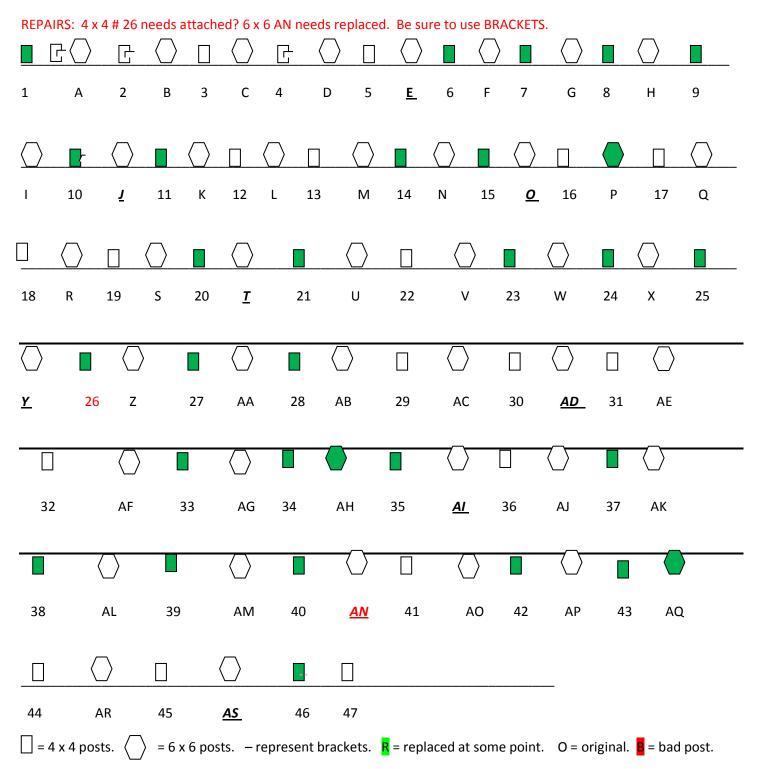
1. For every 6 x 6 post that is replaced be sure to put a bracket on each cross board instead of toe nail.
